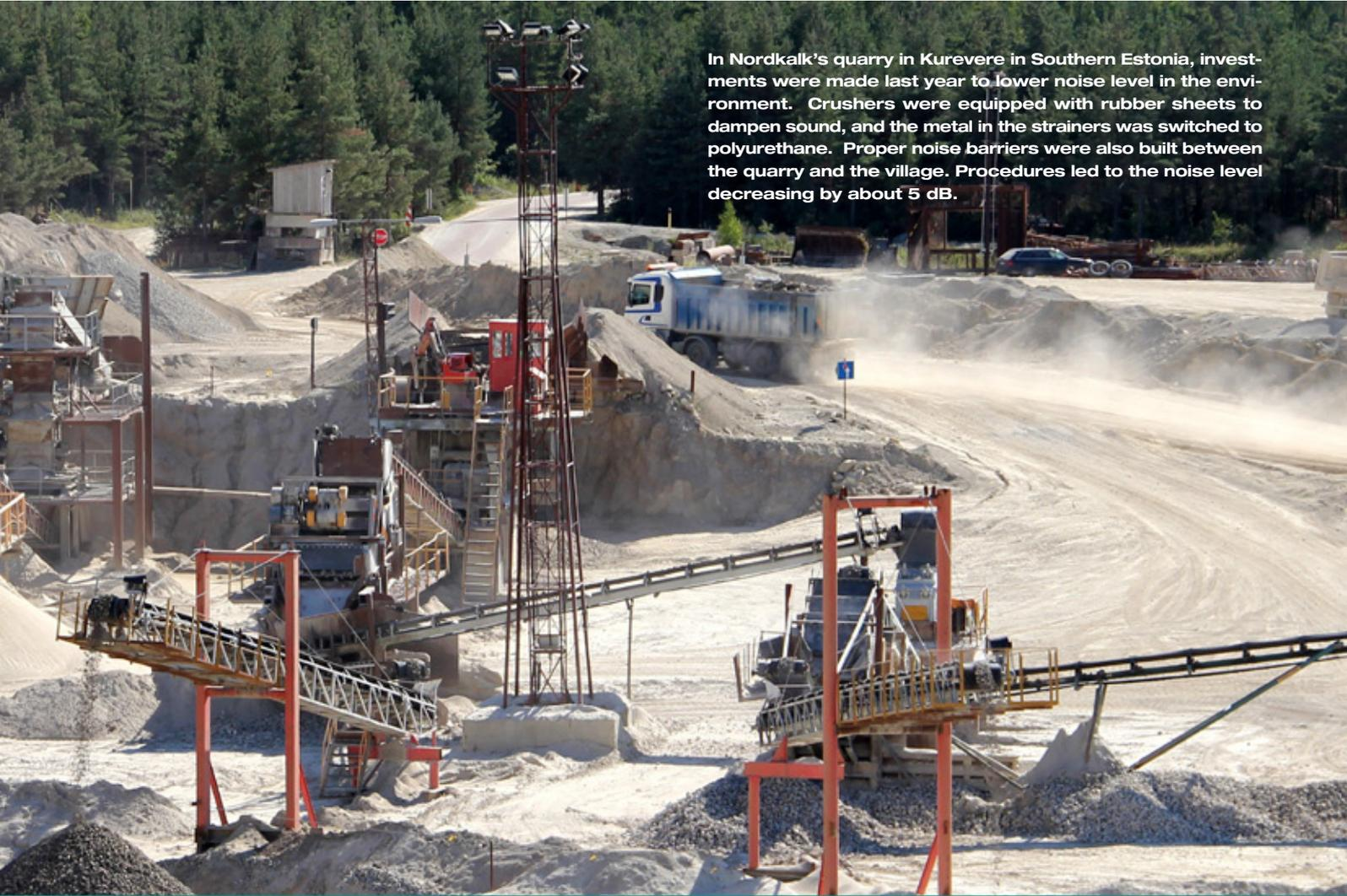
In Nordkalk's quarry in Kurevere in Southern Estonia, investments were made last year to lower noise level in the environment. Crushers were equipped with rubber sheets to dampen sound, and the metal in the strainers was switched to polyurethane. Proper noise barriers were also built between the quarry and the village. Procedures led to the noise level decreasing by about 5 dB.
